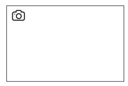
• Video (video recording; the icon ) is displayed in the upper left corner of the display, the total remaining recording time is given taking into account the current resolution in the HH:MM format (hours:minutes).
