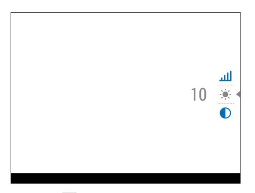
Brightness Totate the controller (6) to change the display brightness value from 00 to 20.
