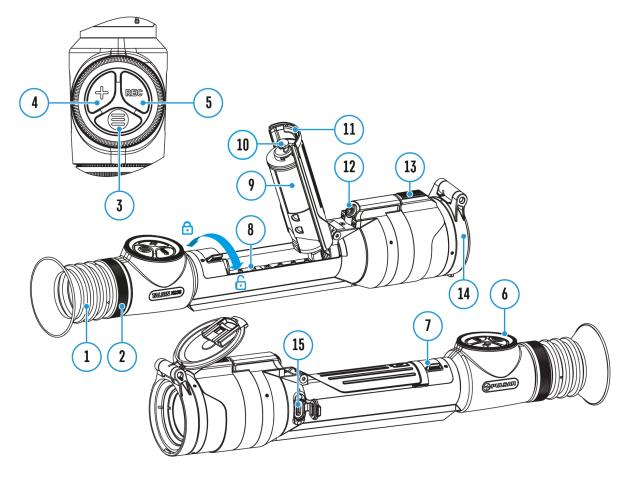
Thermal imaging riflescopes are equipped with a stadiametric rangefinder, which allows you to determine the approximate distance to an object, if its size is known.
