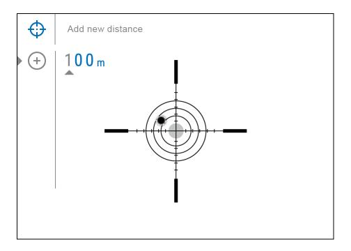
**3.** After adding the distance, it will switch to the **Zeroing parameters settings** menu  $-\frac{1}{1}$ . An auxiliary cross  $\times$  will appear in the center of the display, and X and Y coordinates of the auxiliary cross will appear in the upper right corner.
